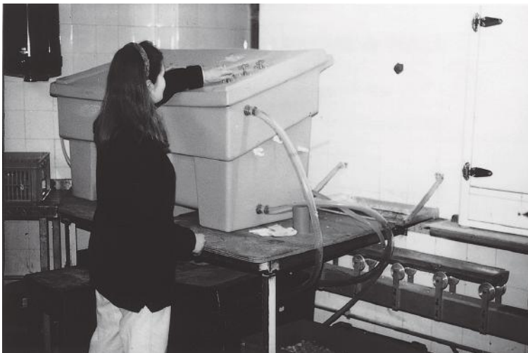
Figure 2.3 In the laboratory: (a) preparation of dinosaur specimens at the Royal Tyrrell Museum of Palaeontology, Drumheller, Alberta, Canada, using a dental drill to remove rock matrix from the bones; (b) Rachael Walker adjusts an automated sieving machine for processing sediment containing microvertebrate remains, designed by David J. Ward, in the Palaeontology Laboratory, University of Bristol, UK. Source: M.J. Benton, University of Bristol, UK. Reproduced with permission.
