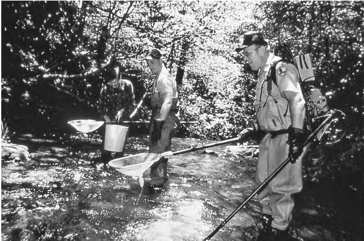
Figure 15.1. Electroshocking temporarily stuns fish so that they can be captured, examined, and then released.
