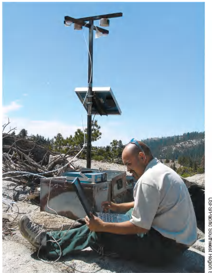
FIGURE 25.17 Air Quality Monitoring in the Sierra National Forest Air samples are collected regularly to monitor temporal changes in air chemistry and particulates. Air quality in national parks and wilderness areas, such as the Sierra National Forest, has been compromised by emissions of pollutants, including \text{NO}_x and sulfate aerosols. These pollutants not only lower visibility, but also pose a health hazard to the organisms that come into contact with them, including humans.
