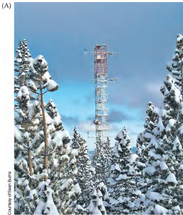
FIGURE 20.9 Eddy Covariance Estimates of NEE (A) A tower projecting above a subalpine forest on Niwot Ridge, Colorado. Instruments attached to the tower measure the microclimate (temperature, wind speed, radiation) and atmospheric CO 2 concentrations at frequent intervals. These measurements are used to estimate net ecosystem exchange of CO 2 . (B) Concentrations of CO 2 (in parts per million) from the ground surface to above the canopy in a boreal forest in Siberia, measured over the course of a 24-hour period in the summer. Average canopy height was 16 m. (B after D. Y. Hollinger et al. 1998. Agr For Meteorol 90: 291–306.)
