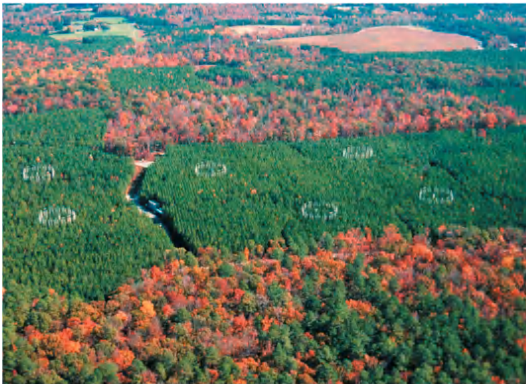
FIGURE 25.4 A FACE Experiment The circles visible in this aerial photo are free-air CO 2 enrichment (FACE) treatment rings in a loblolly pine ( Pinus taeda ) forest in the Duke Forest in North Carolina. Carbon dioxide is released from plastic pipes surrounding treatment plots at a rate calculated to raise the CO 2 concentration to 200 ppm above ambient atmospheric CO 2 concentrations.
