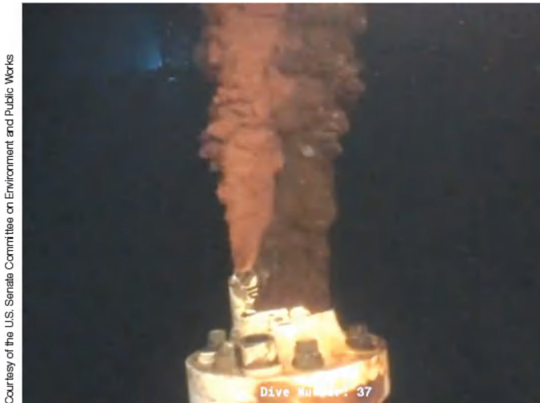
FIGURE 5.19 An Environmental Disaster Oil pours from the fractured wellhead of the Deepwater Horizon oil drilling rig at the seafloor 1,700 m (5,700 feet) below the surface. About 57,000 barrels (9.1 million liters) were released each day for more than 3 months. The impact of this disaster may have been somewhat lessened by the activities of marine microorganisms that were able to use the oil as an energy source.
