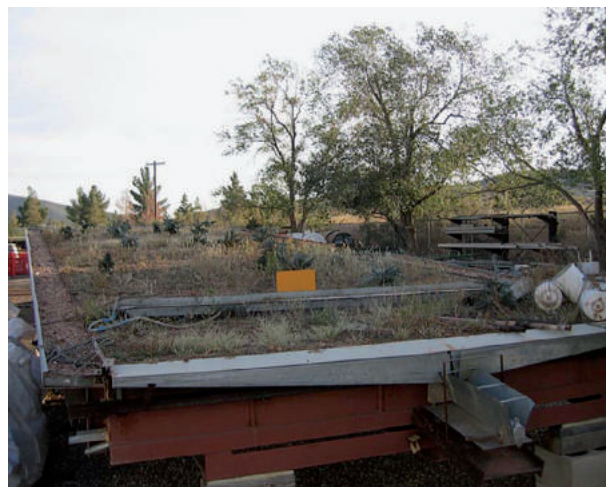
Fig. 2 A platform size physical watershed model (Research Station of the US Department of Agriculture in Tombstone, Arizona).
