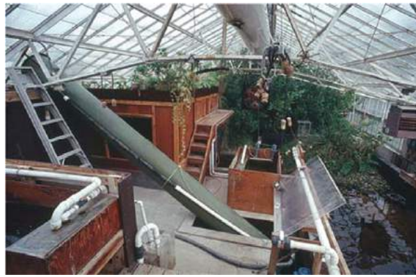
Fig. 3 Engineering/control pad in the Florida Everglades mesocosm. The green diagonal tube in the center is an Archimedes screw that lifts water from the coastal tank (far right) for distribution to the estuary (back right), the ATS (left-foreground), and the wave generator (out of view to lower right).
