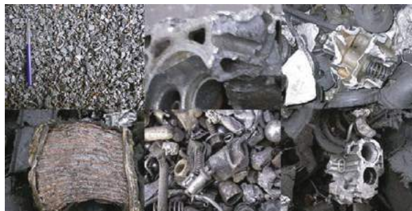
Fig. 6 The ‘mineral’ aluminum in its different appearances (liberation and particle-size classes) as a high-quality liberated fraction (top left) to unliberated radiator (bottom left) and various unliberated mixed fractions that cannot necessarily be recycled directly.
