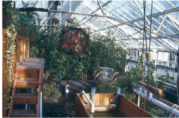
Fig. 2 Red mangrove community in the Florida Everglades mesocosm from the engineering control pad. The large fan in the upper center provides wind for the mangrove communities. The box in the lower right is one of a bank of five algal turf scrubbers (ATSS) that control water quality (nutrients, pH, O 2 ) in the coastal system.
