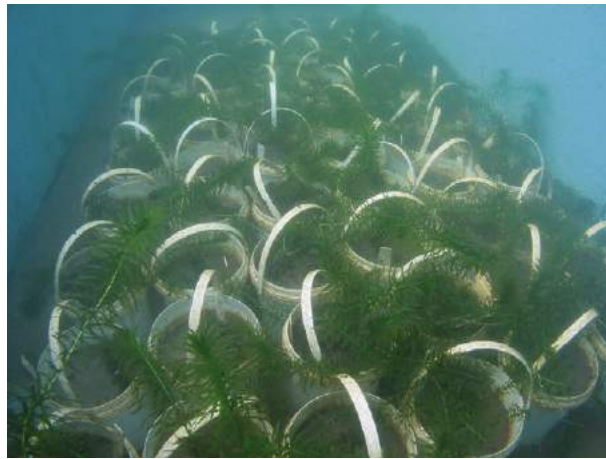
Fig. 4 Simple aquatic microcosms (4 l pails in a 1 m depth flow-through freshwater tank) used to investigate the effects of different sediment types on the growth responses of selected submersed macrophyte species (Matheson et al. ).
