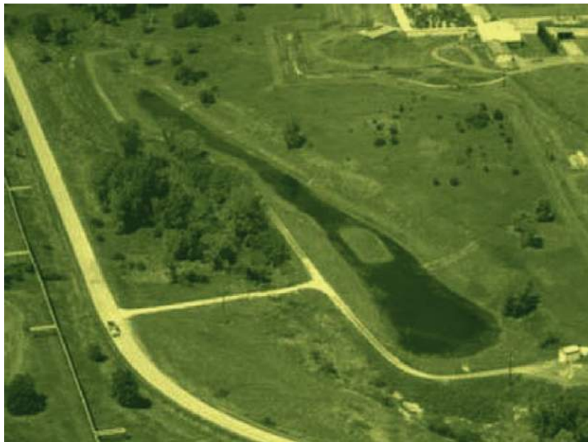
Fig. 3 One of two constructed wetlands at the Iowa Army Ammunition Plant that has zero discharge of TNT and other explosives seeping out of the contaminated groundwater below the explosives manufacturing line shown in the upper right-hand corner. Explosives-contaminated soil was dug up along a stream channel leaving a pit that was then shaped to capture all contaminated groundwater and favor indigenous aquatic plants known to transform explosives. By not having to refill the pit with clean soil, approximately US$ 700 000 was saved. Sediment from local wetlands was used to seed the constructed wetland and provide nutrients. The stream channel was moved to the left as shown to convey less-contaminated stream flow around the wetland. The initial 28 months of monitoring showed elevated explosives concentrations entering the wetland each spring, decreasing in peak concentration the second spring, and dropping to undetectable levels by fall due to plant and algae uptake and transformation. Thorough sampling and analysis established that explosives and the associated transformation products were undetectable and thus did not accumulate in the indigenous wetland plants and algae. The wetland control structure at the lower right of the photograph has never been opened, thus achieving a zero discharge. Evaporation prevents flow out of the wetlands. Slightly more was spent than the US$ 700 000 cost savings and this small difference was due to added monitoring costs of these pilot applications. Thus phytoremediation is not only less expensive, but reduced site restoration costs can also fully offset construction and monitoring costs. Photo courtesy of Kevin Howe, US Army Corps of Engineers, originally and used on the cover of Phytoremediation (2003) Wiley.
