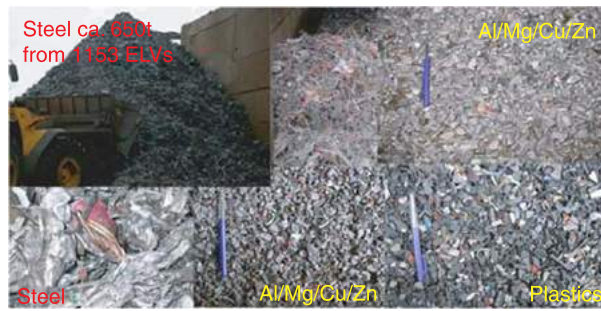
Fig. 5 Impure quality materials created during physical separation of shredded ELVs (clockwise top left: steel, wires, Mg/Al/Zn/Cu/SS, steel/Cu, Mg/Al/Zn/Cu/stainless steel (SS), and plastics). Reproduced by permission of Elsevier.
