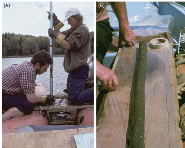
Fig. 3 (A) Coring lake sediments using a Livingstone piston corer at Haugtjern, southeast Norway and (B) a 1 m long, 2.5 cm diameter core of lake sediment extruded from a Livingstone piston corer at Mangrove Lake, Bermuda.
