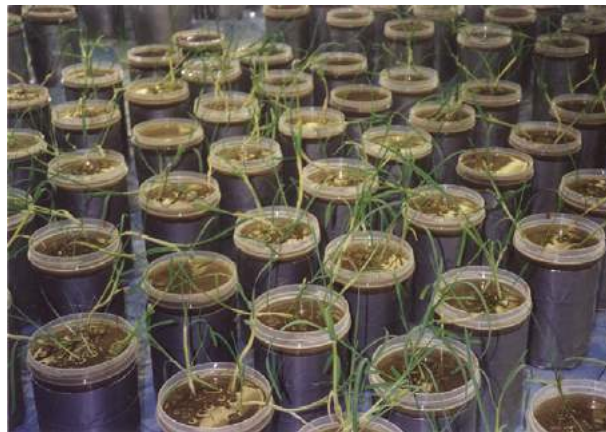
Fig. 5 Riparian wetland soil microcosms set up in a climate-controlled laboratory and used to investigate the fate of nitrate and the effect of wetland plant growth on nitrogen transformation processes (Matheson et al. ).
