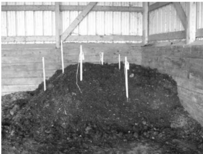
FIGURE 4 Turkey litter composting pile and temperature sensors.
