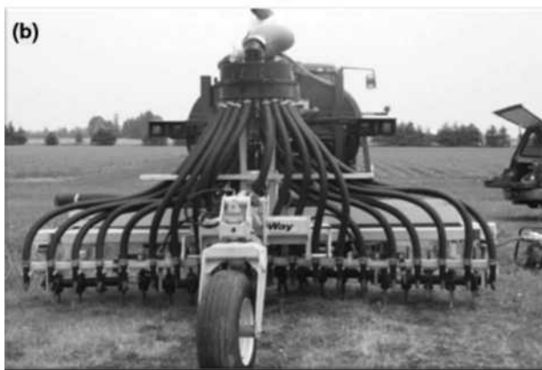
FIGURE 7 Liquid manure injection system: (a) drag-hose system and (b) AerWay SSD system.
