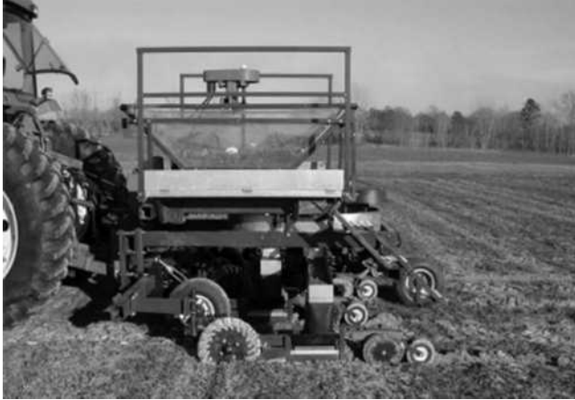
FIGURE 6 Side view of prototype subsurface band applicator implement for poultry litter developed by USDA-ARS at Auburn, Alabama.
