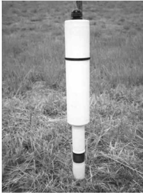
FIGURE 9 A Sensit omnidirectional saltation impact sensor with blue piezo sensing element. The Sensit is mounted vertically by burying the massive base or by inverting the Sensit and supporting the base above the soil surface as shown in the image.
