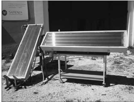
FIGURE 4 Example of an integrated collector storage system.
