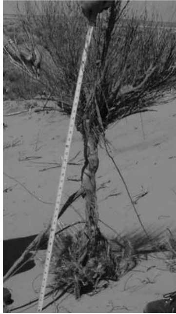
FIGURE 5 Root of a shrub used to measure depth of soil excavated by wind erosion in southern Kansas, the distance to a protected surface (m), and b is the characteristic horizontal length scale or the distance at which f_x = 0.632 f_{mx} . [36]
