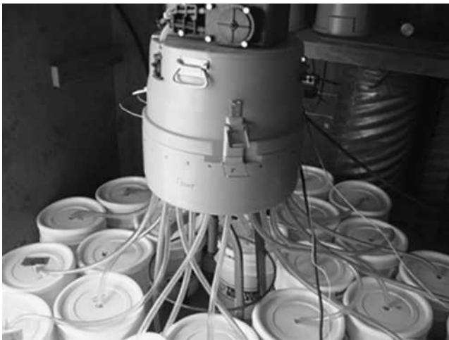
FIGURE 4 Auto-sampler used to collect the water and suspended sediment to determine SSC.
