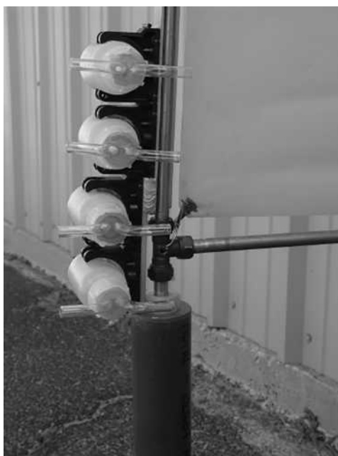
FIGURE 6 A profile of MWAC samplers used to measure the vertical distribution of airborne sediment. Inlet tubes (to the left of the bottles) are oriented into the wind by the sail (to the right of the image) and trap airborne sediment as the mast rotates in the soil mount (at the bottom of the image).
