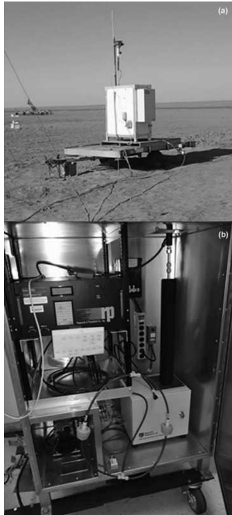
FIGURE 12 A TEOM dust sampler. Air is aspirated through the inlet located above the white enclosure in the field (a) and into a tube before passing through a filter (in the tan base of b). The weight of the filter is periodically recorded by the controller unit (gray panel in upper left of b).
