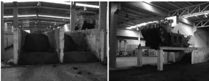
FIGURE 7 Horizontal composting systems: (left) tunnel composting system composed of horizontal parallel beds; (right) turning machine for a tunnel composting system.
