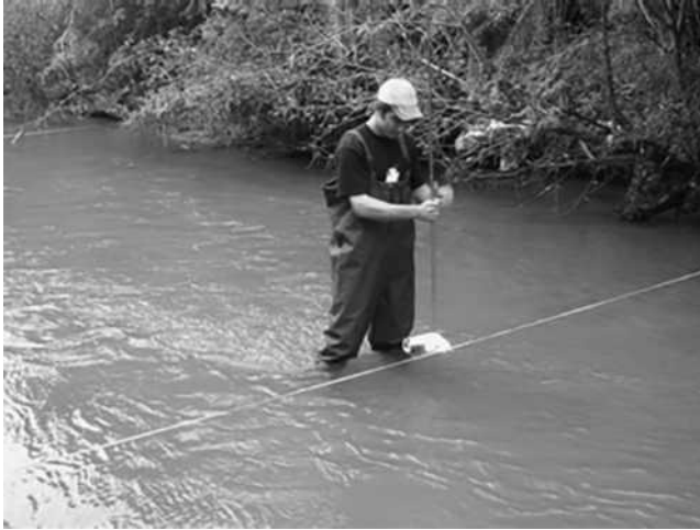
FIGURE 3 Equipment used to collect the water and suspended sediment to determine SSC.
