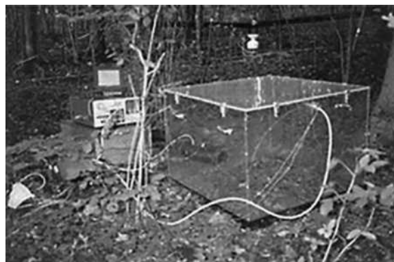
FIGURE 2 Field set-up of an open chamber with removable lid to measure NO fluxes from forest soils: In the front, the outlet with the air sampling tube; in the back, the air inlet with the air sampling tube and the NO analyzer with data acquisition system.
