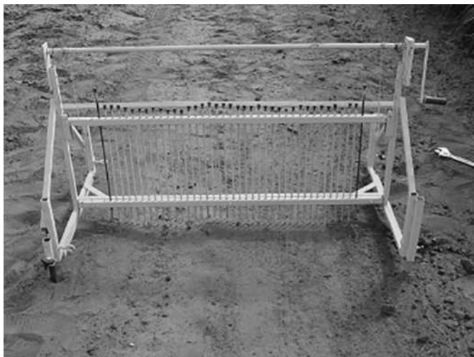
FIGURE 4 Pin frame with pins conforming to the soil surface. Dark pins on both outside edges of the frame are resting on erosion pins.
