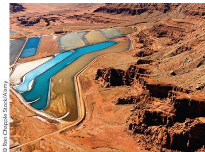
(a) This aerial view shows tailing ponds for mineral wastes, located in Utah.
