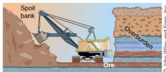
b. Strip mining (surface). Strip mining removes overburden along narrow strips to reach the ore beneath.
