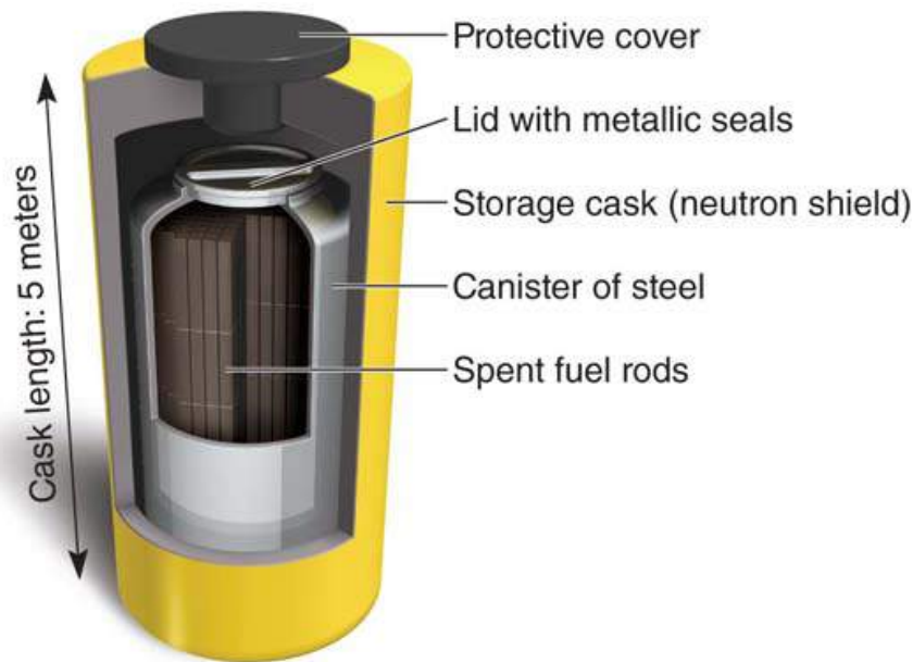
FIGURE 12.19 Dry cask storage for spent fuel
