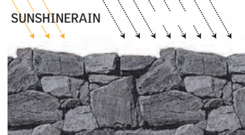
1 Solid rock exposed to the atmosphere begins to weather and erode.
