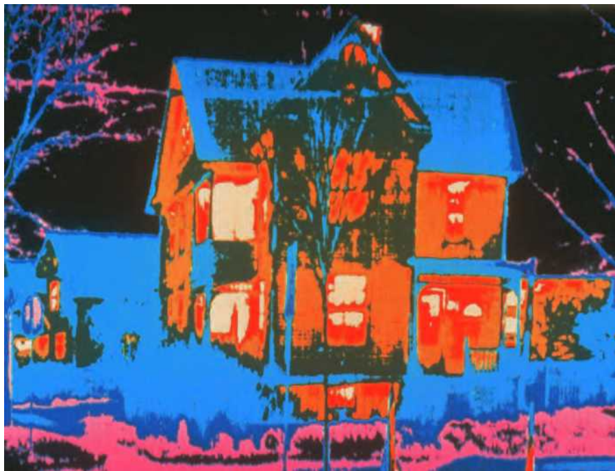
FIGURE 16.1 A thermogram, or infrared photo, of a house that is poorly insulated and poorly sealed and thus loses heat (reddish areas) and wastes money. Critical thinking: How do you think the place where you live would compare to this house in terms of heat loss?
