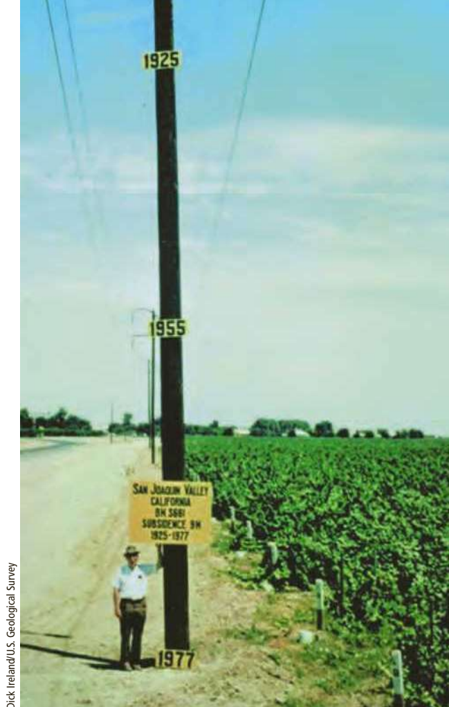
FIGURE 13.13 This pole shows subsidence from overpumping of an aquifer for irrigation in California's San Joaquin Central Valley between 1925 and 1977. In 1925 this area's land surface was near the top of the pole. Since 1977, this problem has gotten worse.
