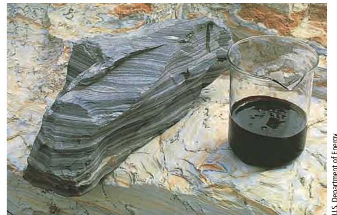
FIGURE 15.7 Heavy shale oil (right) can be extracted from oil shale rock (left).
