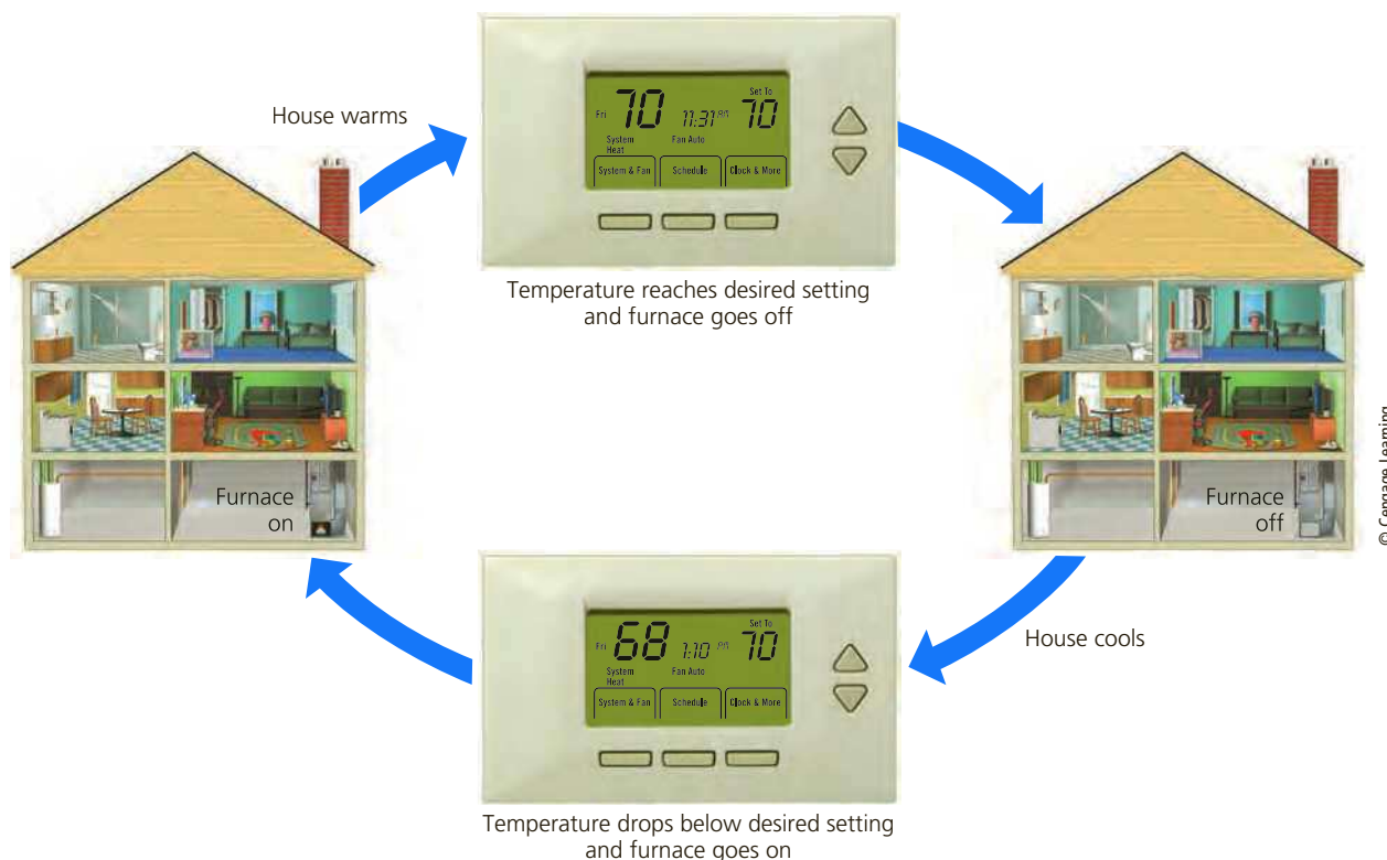
FIGURE 2.16 A negative feedback loop . When a house being heated by a furnace gets to a certain temperature, its thermostat is set to turn off the furnace, and the house begins to cool instead of continuing to get warmer. When the house temperature drops below the set point, this information is fed back to turn the furnace on until the desired temperature is reached again.
