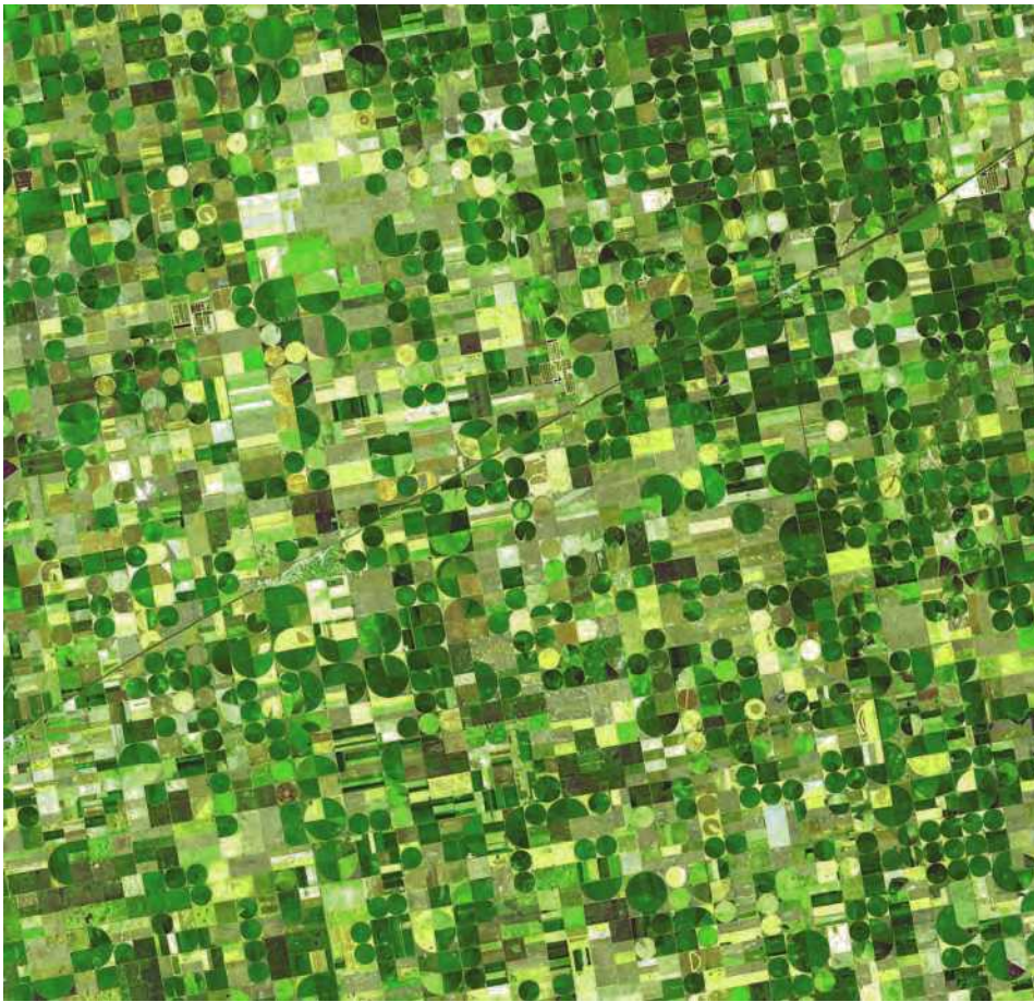
FIGURE 13.12 Satellite photo of crop fields in the U.S. state of Kansas. Center-pivot irrigation uses long, suspended pipes that swing around a central point in each field. Dark green circles are irrigated fields of corn, light green circles are sorghum, and light yellow circles are wheat. Brown areas are fields that have been recently harvested and plowed under. The water used to irrigate these crops is pumped from the Ogallala Aquifer.
